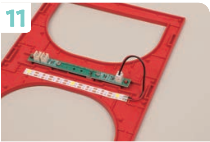
Route the Cable with LEDs as shown, and plug its connector into the socket on the Circuit Board.
